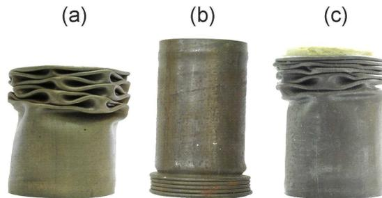
Fig 2. Specimen deformation modes.
